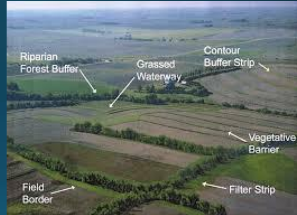
Schematic Illustration of Several In-Field and Edge-of-Field Buffer Types (photo courtesy of USDA-NRCS).
